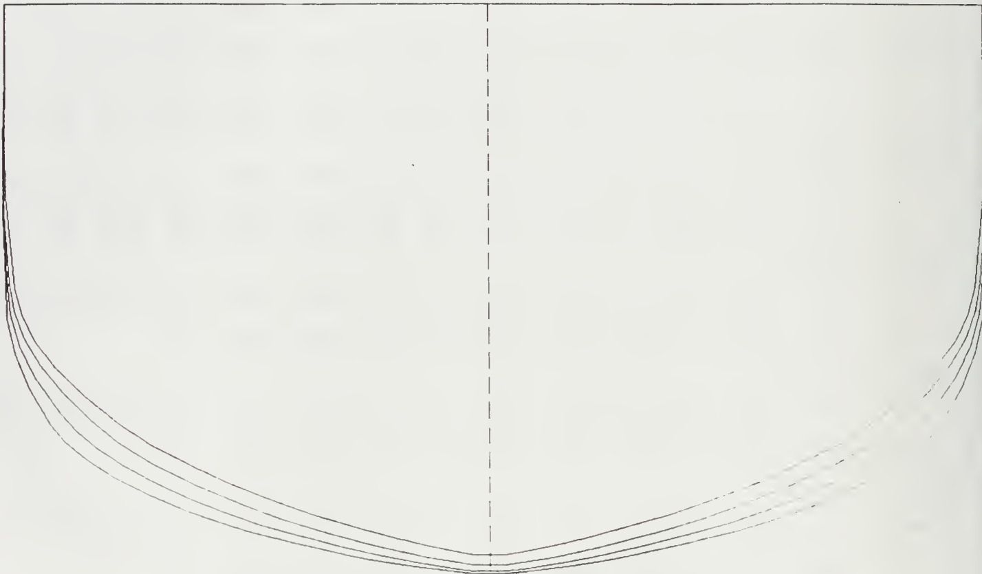
COMP_G.C Body Plan (1 component) Scale = 1:100
